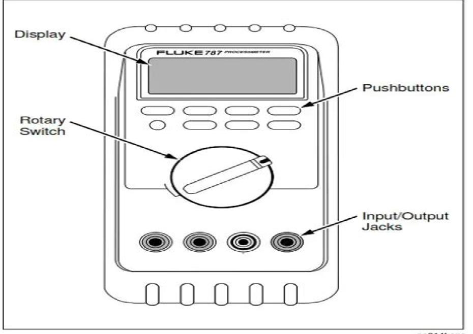
Figure 1. Fluke 787 ProcessMeter
