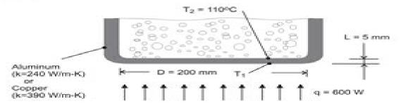
ASSUMPTIONS: (1) One-dimensional, steady-state conduction through bottom of pan.
