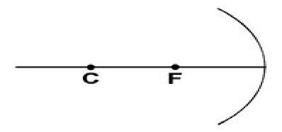
Case 4: The object is located at the focal point (F)
