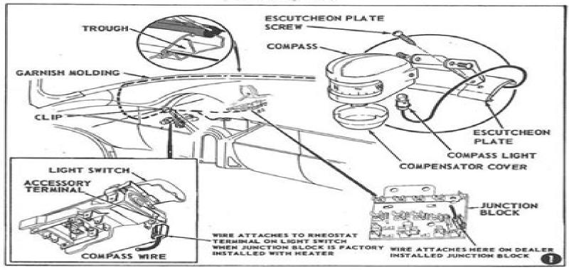
Remove the screw holding the garnish molding escutcheon plate at the center of the windshield. Discord the screw.
