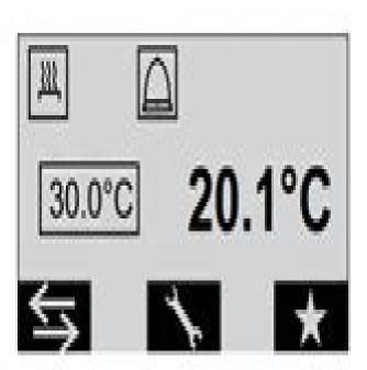
Press to start the bath and display the fluid temperature. If the reservoir fluid temperature is below the set point the heater will start.
