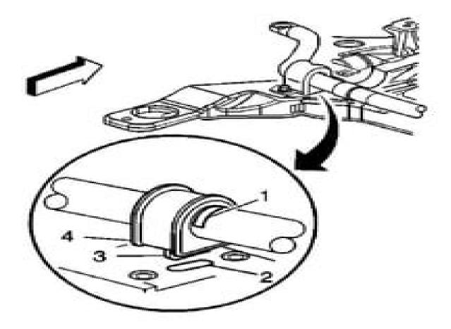
Fig. 8: View Of Left And Right Stabilizer Shaft Insulators And Brackets Courtesy of GENERAL MOTORS CORP.
